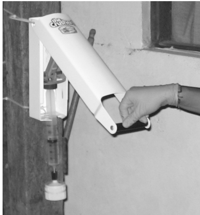
Figure B1. Modified can crusher used with sterile syringe and filter holder. Craig Carlson is acknowledged for the idea and design. Guy Grant is acknowledged for the modification of this can crusher.
